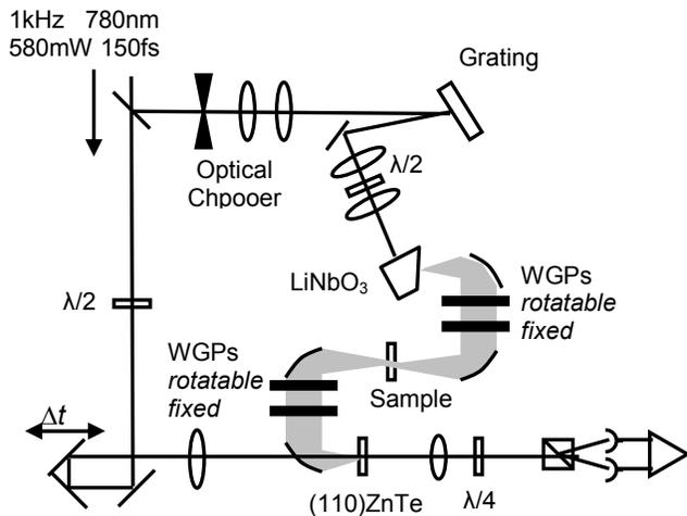
Fig. 1: Experimental setup of THz nonlinear transmission spectroscopy
