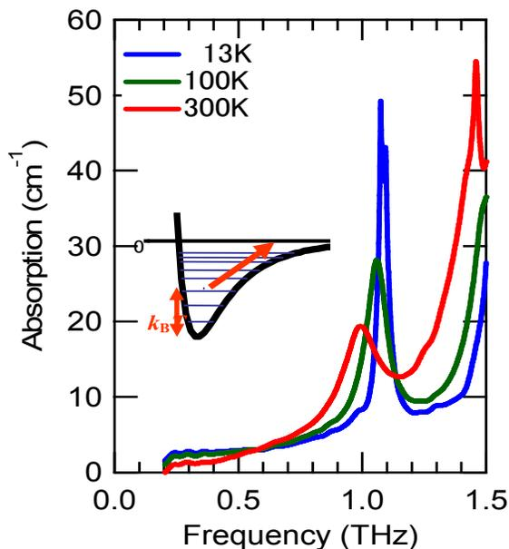
Fig. 3: (a) Linear absorption spectra of L-arginine pellet at 13 K, 100 K, and 300 K,
