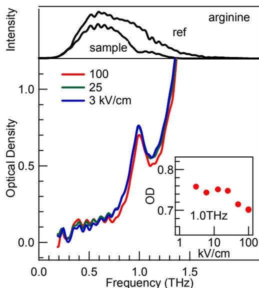
Fig. 4: (a) Power spectrum of the transmitted THz wave and the reference THz wave. (b) Optical density at different electric field amplitude at 300K
