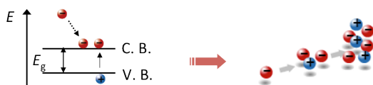
Fig. 3: The sketch visualizes the impact ionization process, where an electron loses its kinetic energy and an electron-hole pair is created simultaneously. A significant number of electron-hole pairs are generated by a series of impact ionizations.
